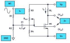
Figure 1. Common source amplifier test configuration.
