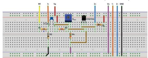
Figure 2. NMOS diode breadboard circuit.
