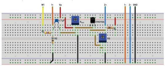
Figure 5. Source degeneration added to a breadboard connection.
