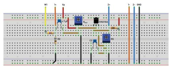
Figure 8. Breadboard connection with C2 added.
