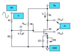
Figure 7. C2 added to increase ac gain.
