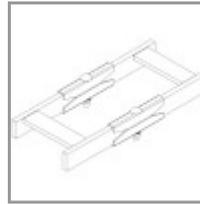
Easy-to-use butt-splice kit safely and securely connects 2 sections of cable management ladder end-to-end.
