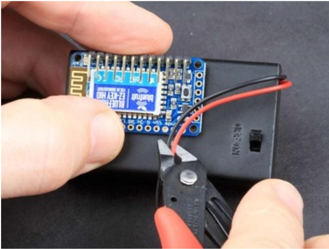
Position the EZ-Key on top of the battery holder as shown. Measure and cut the wires so they are just long enough to reach the Vin and Gnd holes on the board.
