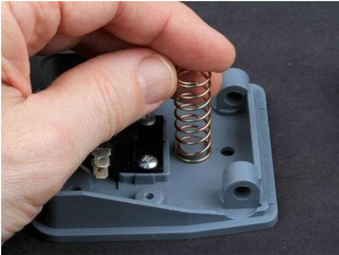
Position the spring between the two halves of the foot switch.
