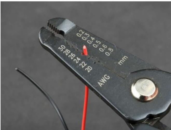
Strip the wires and solder them to the Vin and Gnd holes.
