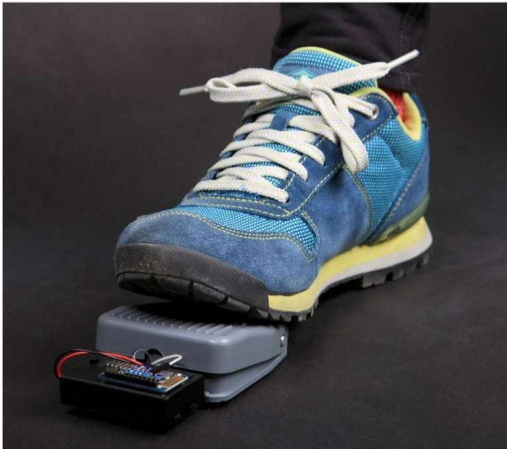
This is a quick and easy project that will speed your work on future projects. By combining an Adafruit BlueFruit EZ-Key with a foot switch, we end up with a wireless, hands-free scroll button. No need to put down that hot iron to see the next step in the tutorial. Just give the pedal a tap with your foot to scroll down the page.
