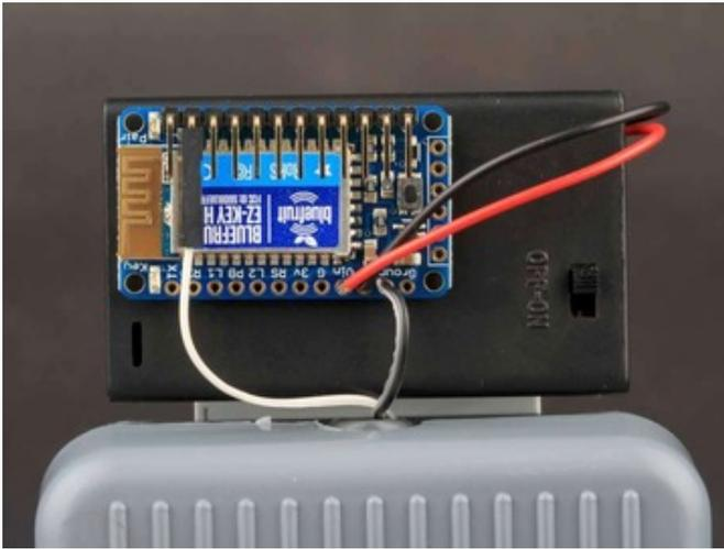
Connect the jumper to pin #1 of the right-angle header.
