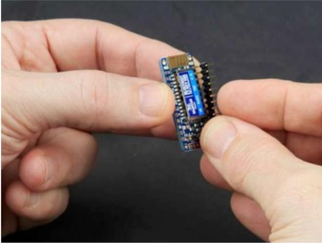
Cut a 12-pin section from the right-angle header strip and solder it to the holes marked 0-11.
