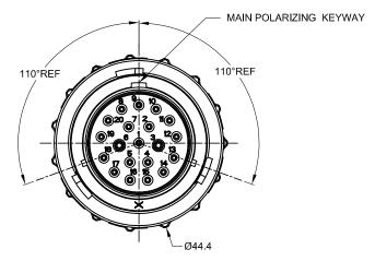
PLUG, 18-20 POS, PIN CONT., REDUCED DIA. SEAL, AHDP
